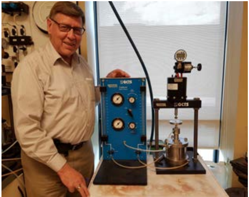
Fredlund designed a new pressure-plate testing device for GCTS that can apply soil suctions up to 1,500 kPa and Ko total stress loading, and continuously monitor overall volume changes and water volume changes.
